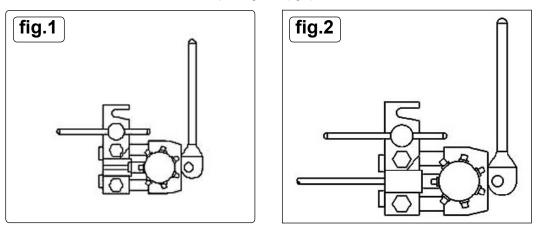
4.1.8. After the pipe has been prepared as instructed above, ensure the tube nut is fitted to the pipe. Pass the pipe through the rear of the die until the prepared end is flush with the front face of the die. Ensure that both halves of the die are contacting the die stops (fig.2). Swing the locking plate into position and tighten the clamping screw. Check that the position of the pipe and die are still correct.
